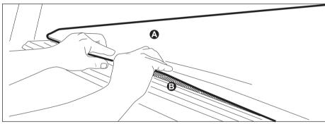
7. Please check whether the tarp is closing with the Velcro on the rails tightly and horizontally, then the installation is finished.
