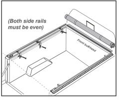
3. Put one side rail (B/C) on the truck bed and slide into the channel of cover assembly (A), then tighten the set screws on the both corners to secure the connection, do the same way for the other side.
