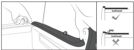
1. Wipe and clean the tonneau before installation. If there is a drop between the front and side of bulkhead, sticking the seal strip(D) to the front bulkhead and align both ends equally.
