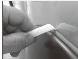
Place the edge trim against vehicle by hooking curved end beneath edge trim at one end of flare and then slide the outer edge of flare to the other end with the provided Edge Trim Tool.
