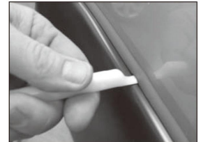
Place the edge trim against flare by by inserting straight end between edge trim and flare at one end and then slide around entire edge to the other end with the provided Edge Trim Tool.
