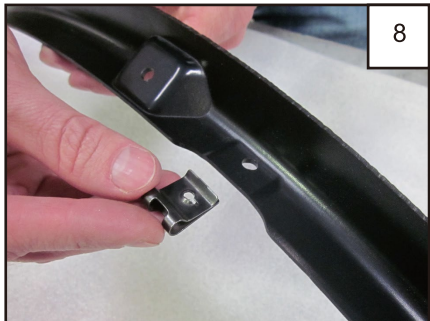
Verify presence of U-clip on inner brackets.
