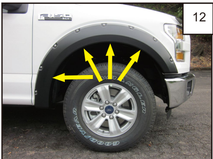
Position flare on fender, pressing inward on the flare, line up the flare mounting holes with the mounting clips on the inner piece. Install four Phillips Truss Screws (SW1-0058) through the flare and into the clips on the inner piece. Install and tighten.
