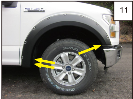
Hold flare to fender, re-install three factory screws removed in Step 4 using sockets and wrench.
