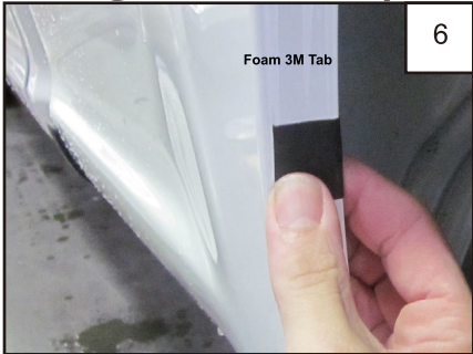
Wrap a Foam Tab (MT1-0014) around the wheel well sheet metal, centered over the mark made in Step 5.
