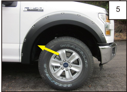
Hold flare to vehicle and mark one flare hole location with a grease pencil.
