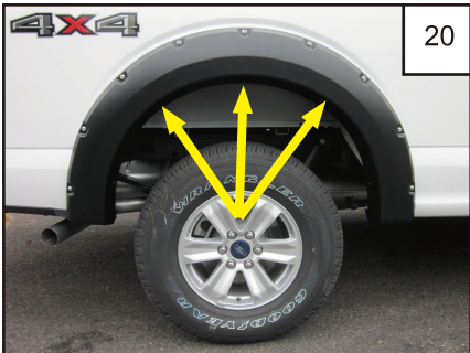
Press flares firmly onto the vehicle and install and fully tighten three screws (SW1-0050) into the clips installed in step 18.
