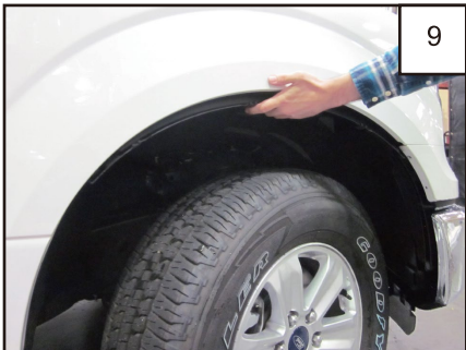
Line up the holes in the inner piece with the three uppermost factory holes. NOTE: Both inner brackets are universal.
