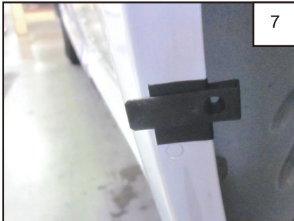
Install a Clip (CL1-0009) over the Tab (MT1-0014) placed in Step 6.
