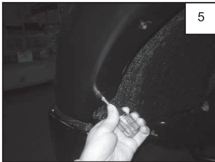
Using a #2 Phillips Screwdriver, install two supplied Tufloks (RV1-P001) through additional holes in flare and into fender. NOTE: Use a push-twist motion.
