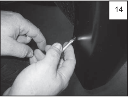
Install four supplied Screws (SW1-0050) through remaining holes and into clips installed in Step 12, working from front to back of wheel well.
