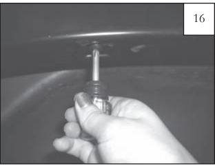
Reposition flare on fender, Start a supplied Screw (SW1-0057) through the two uppermost holes in the flare and into each Clip installed in Step 11.
