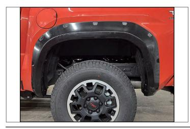
Using supplied Edge Trim Tool, seat edge trim against vehicle by hooking curved end under edge trim at one end of flare. Next, slide around outer edge of flare to the other end.
