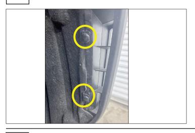
Remove flare by pulling part away from side of vehicle
