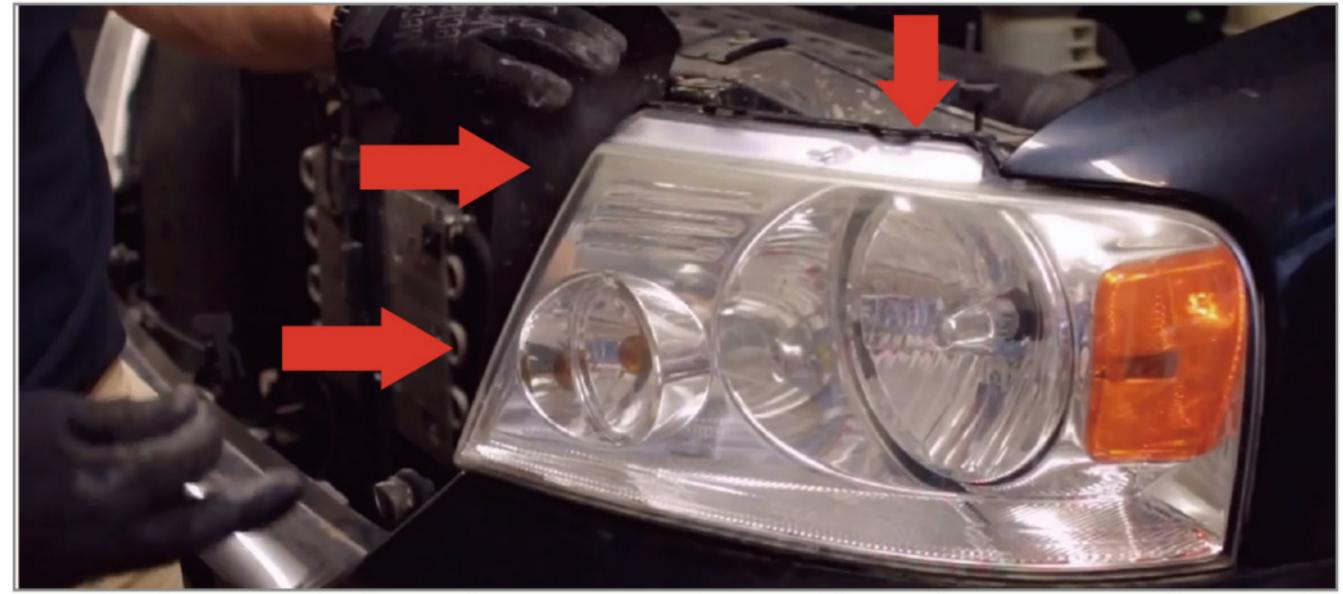
Pull the quick release tab on fender panel. Crab the corner on fender side and pull the headlamp off from the vehicle.
