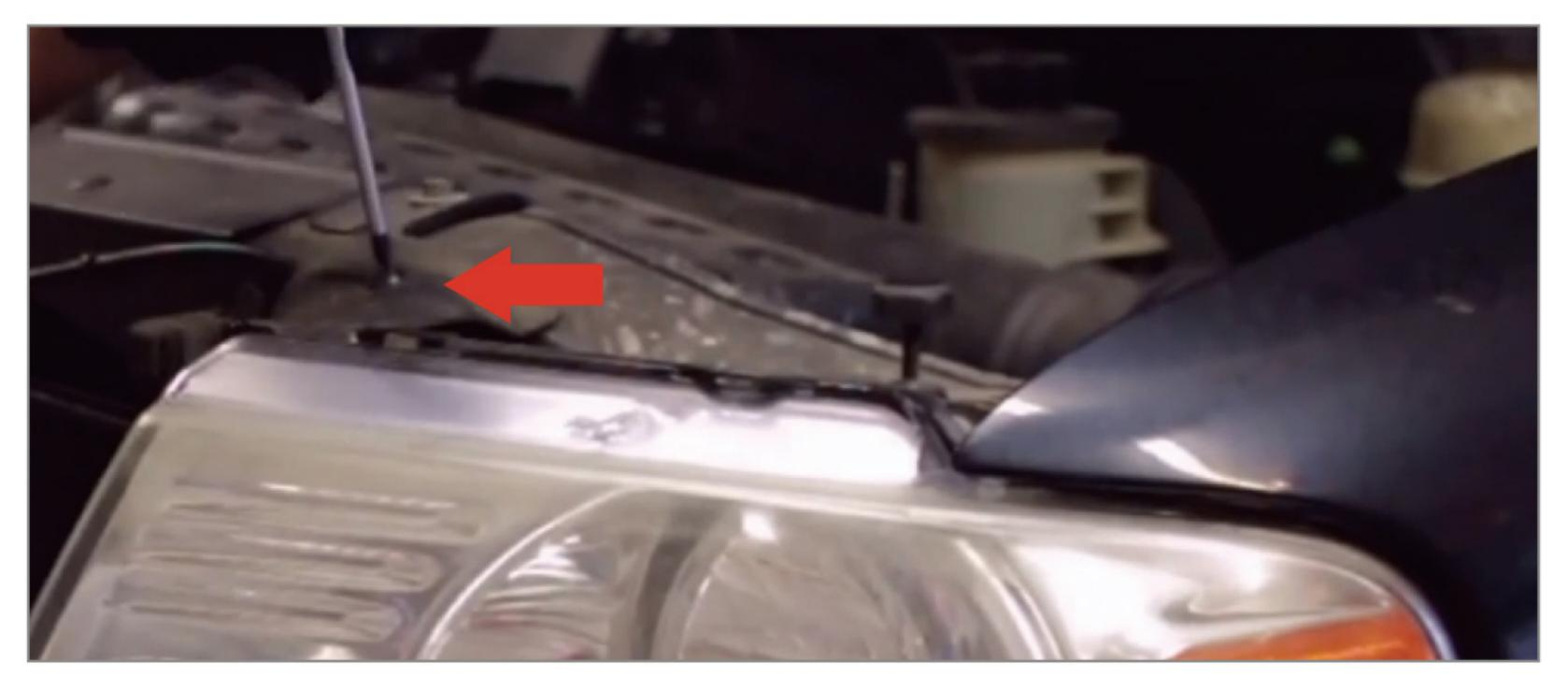
Pull off the rivet and keep weather shield away from headlamp.
