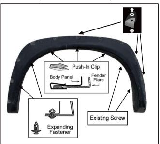
Use allen key to tight allen bolt ,washer & nut firmly on ever pocket of the fender flares first , then place the flare on the vehicle with best position. Apply 3 Push-In Clip into the mounting slot in flare and secure it to the vehicle. Apply 2 Plastic Expanding Fastener into the mountin g slot in flare and secure it to the vehicle as shown. Fasten the existing factory screws into the original location that were previously removed.
