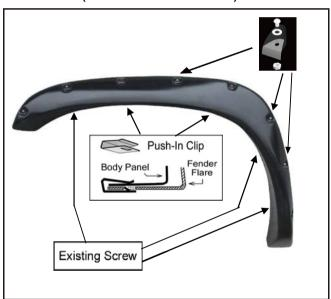
Use allen key to tight allen bolt ,washer & nut firmly on every pocket of the fender flares first then place the flare on the vehicle with best position. Apply 2 Push-In Clip into the mounting slot in flare and secure it to the vehicle as shown. Fasten the existing factory screws into the original location that were previously removed.
