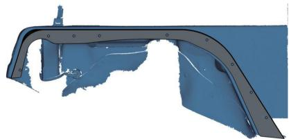
3. Secure the front fender flare on body panel with (9) M5×15 drilling screws.
