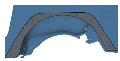
3. Secure the rear fender flare on body panel with (8) M5×15 drilling screws.
