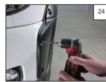
Drill through holes in bumper piece and into sheet metal with a 5/16" drill bit
