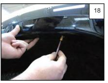
Hold the fl are fi rmly on the fender. Using a grease pencil, mark two clip locations using existing holes in fl are. See step 19
