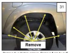
Remove fi ve factory screws. Remove fl are by pulling part away from side of vehicle.
