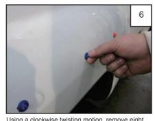
Using a clockwise twisting motion, remove eight factory plastic clips from fender. See step 8.
