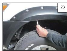
Install a supplied Phillips Truss Screw (SW1-0050) through holes in fl are and into Clips installed in Step
