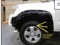
Reposition fl are on fender and install three 20mm hex screws (SW1-0036) through holes in fl are and
