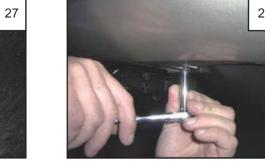
Pull down bumper cover and slide splash shield back in place. Install supplied hex screw (SW1-0036) in front of bumper cover to fasten splash shield to
