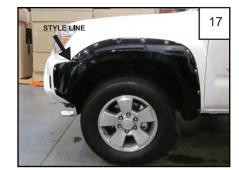
Hold the fl are fi rmly on the fender. Make sure to line up the fl are and bumper piece along the style line to ensure correct installation.
