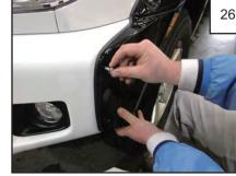
Slide a supplied .320 SS Washer (WA1-0012) onto a SS Torx Screw (SW1-0041). Situate fl are on bumper, inserting screws through holes drilled in bumper in
