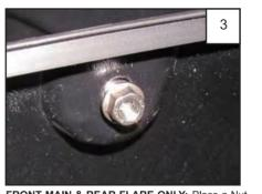
FRONT MAIN & REAR FLARE ONLY: Place a Nut (NU1-0019) over the end of each Bolt and tighten, using a 1/2" wrench for the Nut and the supplied Torx Bit (SW1-0052) for the Bolt. Repeat for remaining
