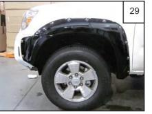
Tighten all screws. Completed Front Flare installation
