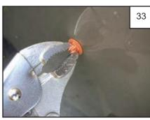
Remove three clips from fender using vise grips, pulling with a rocking motion. See step 34.
