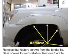
Save screws for reinstallation. Remove fl are by pulling part away from side of vehicle.
