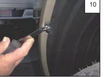
Remove plastic screw located at front of wheel well by turning clockwise 1/2 turn with a fl at head screwdriver and prying out.
