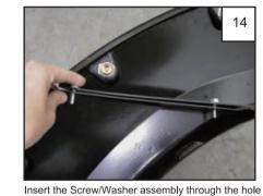
drilled in the end of the Front Main Flare and into the corresponding hole in the Front Bumper Piece. Two
