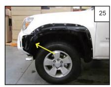
Make sure bumper piece is aligned with the style line. Install supplied 20mm hex screw (SW1-0036) into factory hole on front bumper and tighten.
