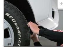
Pull down bumper cover and splash shield. NOTE: Do not re-fasten splash shield until fi nal step.
