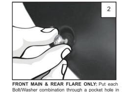
the flare, Bolt head and Washer on the outside.
