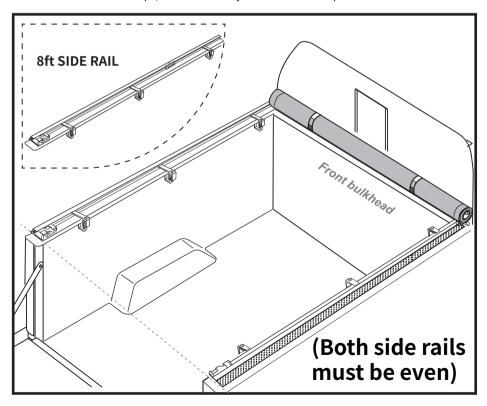
Make sure the side rails are placed so that the distance from the tailgate is equal on both sides.
