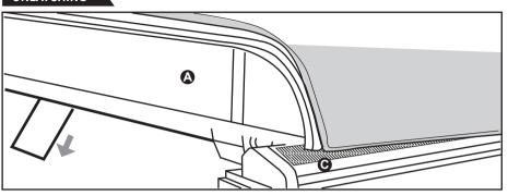
8. Pull the strap to release the rear latching, then roll up the cover from the tailgate towards the bulkhead, and lock the buckles on the cover assembly.
