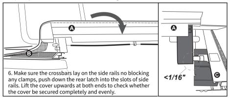
Please ensure the gap between the locking clip and the side rail at end of the tailgate is less than 1/16" for proper security of the cover.If too large,need to adjust the side rail position.
