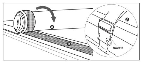
5. Release the buckles on the both sides of cover assembly, then unroll the cover completely from the bulkhead towards the tailgate.
