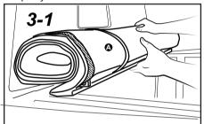
3-1. Place the cover assembly (A) on the bulkhead in front of the truck bed.
