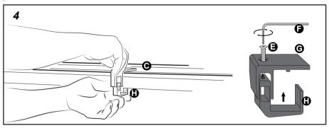
4. Please insert the lower clamps (H) into the truck bed rail lips, and tighten the hex socket screws for the two clamps,do the same way for the other clamps.
