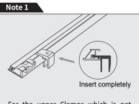
For the upper Clamps which is not pre-installed in the side rails, Please take out those upper clamps from the hardware box and insert into the side rails channel before step 4.
