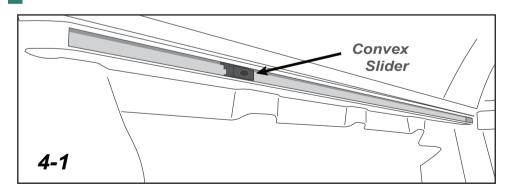
4-1. Insert convex slider into the utility tracks (on both sides of the tonneau).
