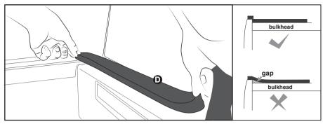
1. Wipe and clean the tonneau before installation. If there is a drop between the front and side of bulkhead, sticking the seal strip(D) to the front bulkhead and align both ends equally.
