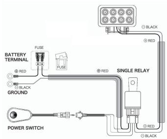
Wiring diagram, the harness not include.
